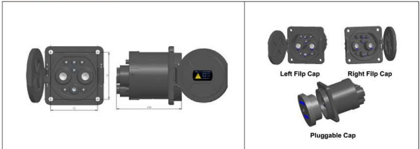
[DC Charging Socket Drawing]
